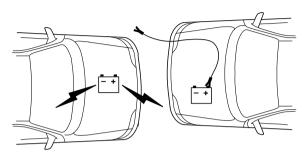
1. Connect the positive (+) booster cable to the positive (+) terminal of the discharged battery.
